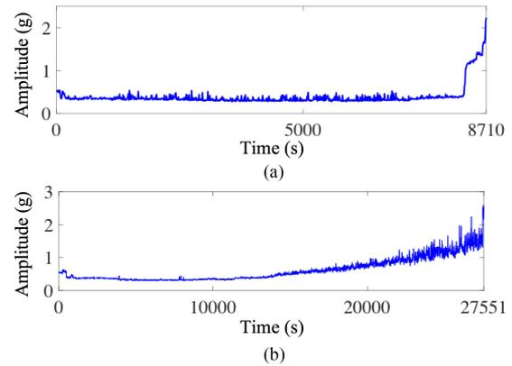
Fig. 3. RMS of two degradation patterns. (a) Sudden degradation. (b) Slow degradation.
