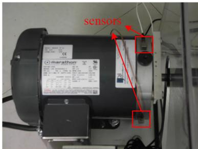
Fig. 8. Locations of two accelerometer sensors.
