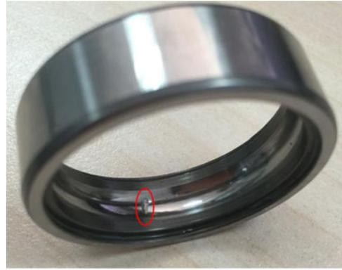
Fig. 13. Defect on the outer race of the experimental bearing.
