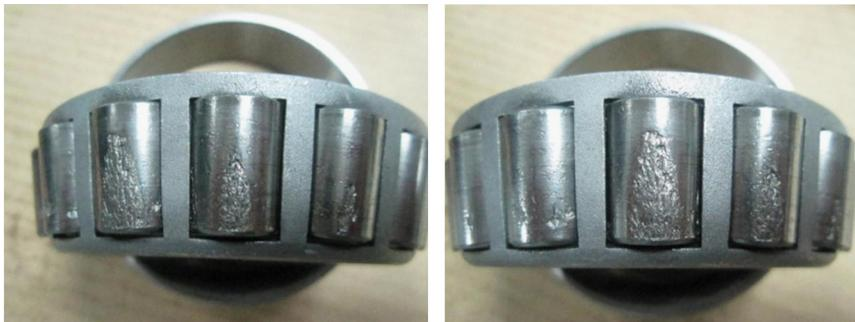
**Fig. 35.** The defects of the failure bearings.
